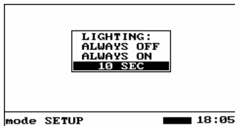
Figure 14. Illumination control panel
